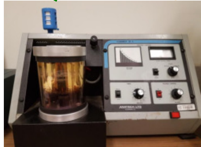
Hummer VI-A gold sputtering device from Anatech LTD
